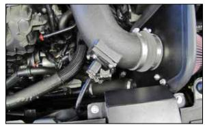
19. Reconnect the Inlet air temperature electrical connection.
