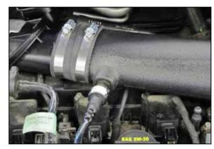
20. Connect the EVAP vent line to the auick disconnect fitting installed into the K&N® intake tube.
