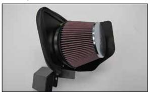
11. Install the K&N<sup>®</sup> air filter onto the filter adapter and secure with the provided hose clamp. NOTE: Drycharger® air filter wrap; part # 22-8049DK is available to purchase separately. To learn more about Drycharger® filter wraps or look up color availability please visit http://www.knfilters.com®.
