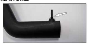
17. Install the provided quick disconnect fitting into the K&N® intake tube as shown.
