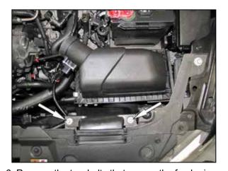
6. Remove the two bolts that secure the fresh air duct to the core support then lift up and remove the complete air filter housing from the vehicle. NOTE: K&N Engineering, Inc., recommends that customers do not discard factory air intake.
